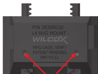
INSERT .050 HEX DRIVER TO ADJUST; CCW TO LOOSEN, CW TO TIGHTEN
